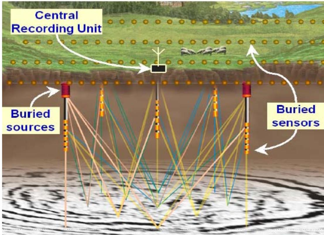
**Figure 1: Seismic monitoring system with five sources, five vertical and four horizontal antennae of receivers.**
