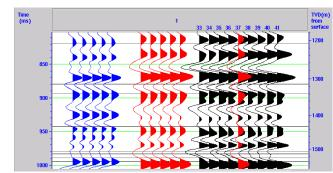
Figure 8. Correlation of synthetic seismic trace and migrated seismic data with spectral color correction. Blue: synthetic seismic trace; Red: migrated seismic trace with CDP 37; Black: migrated seismic traces around CDP 37.
