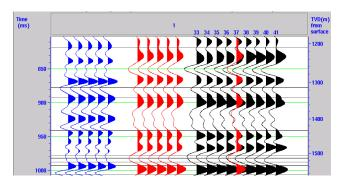
Figure 7. Correlation of synthetic seismic trace and migrated seismic data with plain Gabor decon. Blue: synthetic seismic trace; Red: migrated seismic trace with CDP 37; Black: migrated seismic traces around CDP 37.
