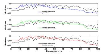
Figure 6. The average amplitude spectra of the seismic data (CDP 50-250, time: 500ms-1500ms) shown in Figure 10 Figure 11 and Figure 12 and the amplitude spectrum of the synthetic seismic trace shown in Figure 1.
