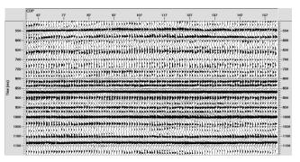
Figure 4. Migrated seismic data with spectral color correction (zoomed).
