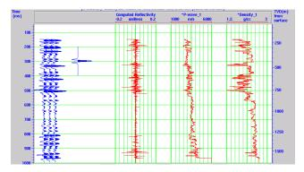
Figure 1. Well log 1409. From left to right: synthetic seismic trace, Ricker wavelet with a dominant frequency of 40Hz, computed reflectivity, P wave velocity and density.
