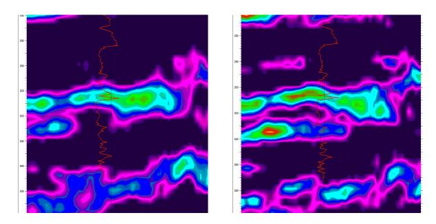
The second facility is the programs in the workstation that allow the identification of various attributes. The simplest of these is just the straight amplitude display. The trick is in the way the amplitudes are displayed. If reservoir attributes change by only 10% of the overall amplitude, then the entire colour range for display should be limited to this 10% range. If there is a statistically significant change of amplitude within the data,
