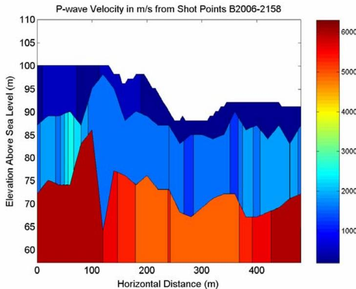
Figure 1: Section of the tomography model used to perform static corrections, showing a layer of top soil, a layer of glacial till, and the underlying schist
