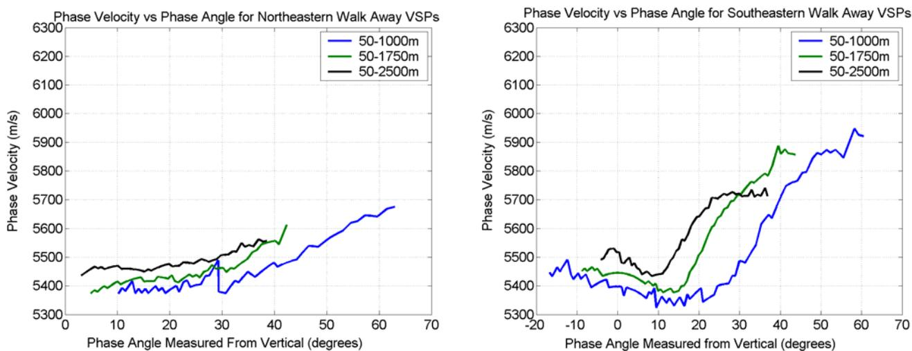
Figure 3: Phase velocity vs phase angle measurements along two different azimuths at the three different depth intervals.
