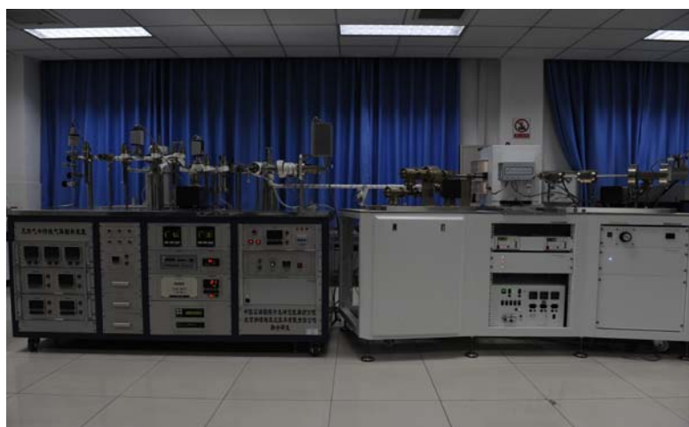
Fig.1 The noble gas sampling system and its isotope mass spectrometer
