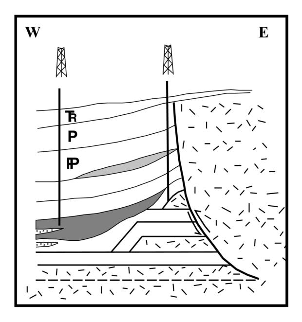
Figure 1. Diagrammatic representation of interpreted thrust duplex comprising two horses beneath the Wolfcampian Uncompanier thrust fault in the vicinity of Uravan, Colorado. Clastic wedges (shaded) that prograded west into the Paradox basin document the age of thrusting as Middle to Late Pennsylvanian.
